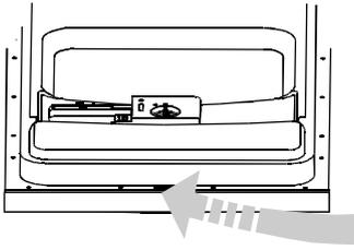
To clean the edge around the door, you should use only a soft cloth and warm soapy water. To prevent penetration of water into the door lock and electrical components, do not use a spray cleaner of any kind. Also, never use abrasive cleaners or scouring pads on the outer surfaces because they will scratch the finish. Some papers towels can also scratch or leave marks on the surface.
